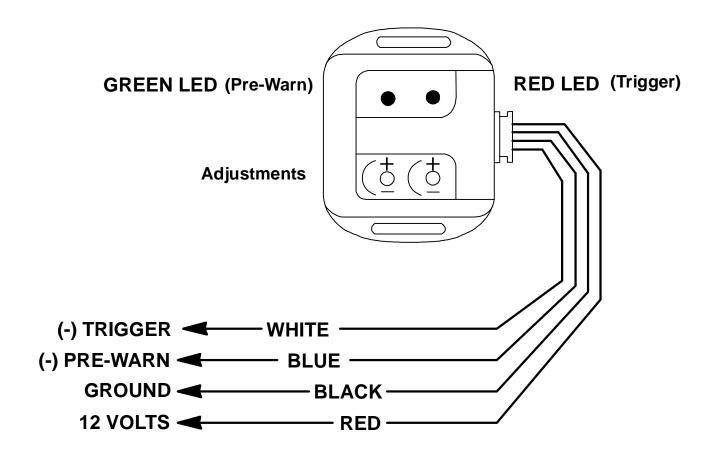
SHOCK SENSOR: The sensor supplied with this system does not require any additional wiring. Simply mount the sensor in a suitable location, plug it in, and adjust for sensitivity.
